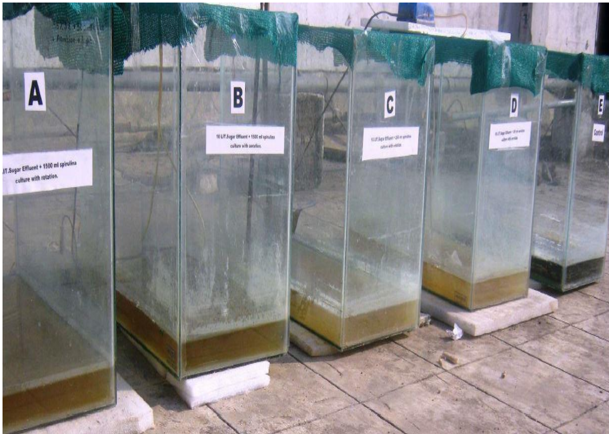
Treatment of industrial effluent using Open type bioreactor (3 rd July 2019)
